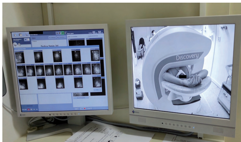
Figure 5 Semiconductor cardiac gamma camera “Discovery CZT 530c” by GE (Central Military Hospital – University Hospital Ružomberok).
