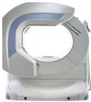
Figure 4 Cadmium–zinc–telluride semiconductor detector. In digital semiconductor gamma cameras with direct gamma radiation conversion, one aperture on the collimator corresponds to one semiconductor detection unit and simultaneously to one resulting image point (pixel).
